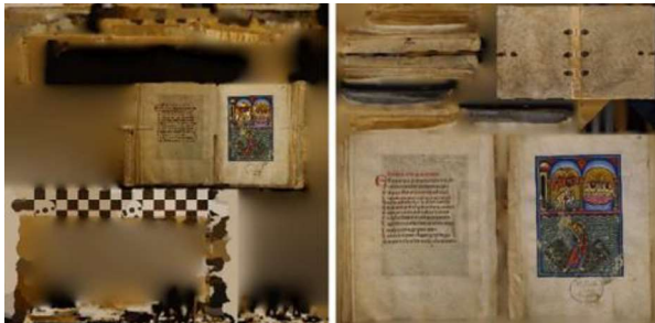
Fig. 3 - Atlas texture created in photogrammetry software using texture building algorithms. Left) texture built using automatically generated texture coordinates; right) texture built using manually created texture coordinates. In the image in the right side the detail was weighted by prioritizing the pages.
